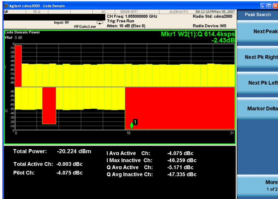
Figure 7-5 Code Domain Measurement Result - Power Graph & Metrics View - Uplink (MS) Peak Marker
